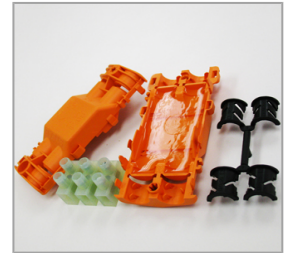
Ordering Code: 9-0904-00 Gel-Filled IP68 Connector for Through Wiring Cable Diameter 6.5 - 12mm.
